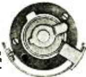
Right: Mechanism showing shoe in contact with ring.
